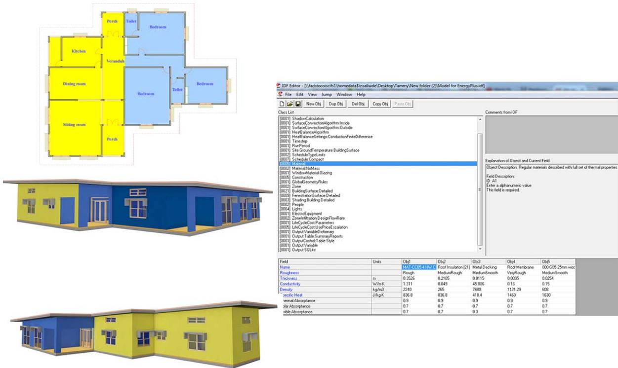
Figure 3: The schematic model and floor plan highlighting zones 1 and 2
