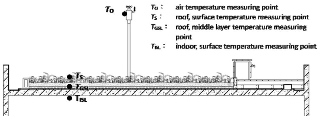
Fig. 1. Position diagram of measuring point
