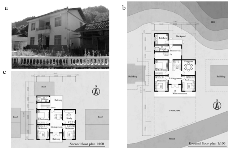
Fig. 3. A contemporary rural house in the Caobachang village of Ningqiang county (a) front yard view; (b) ground floor plan; (c) second floor plan
