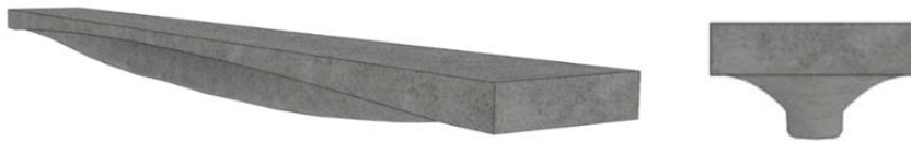
Fig. 4. (Left) perspective view of FAB, (Right) mid-span cross-section
