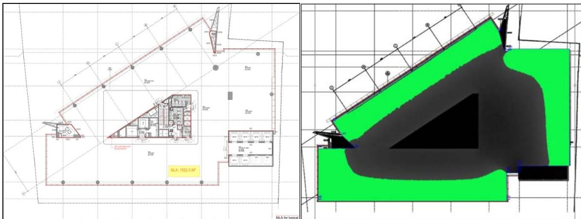
Fig.4. Highrise floor plan and daylight simulation results demonstrating 47.1% of area achieving > Daylight factor of 2.5
