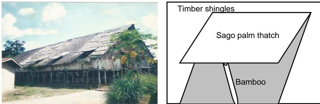
Fig.4. (a) The Merian Bedup longhouse and the *kamban*, the opening on the roof; (b) The *kamban* details.
