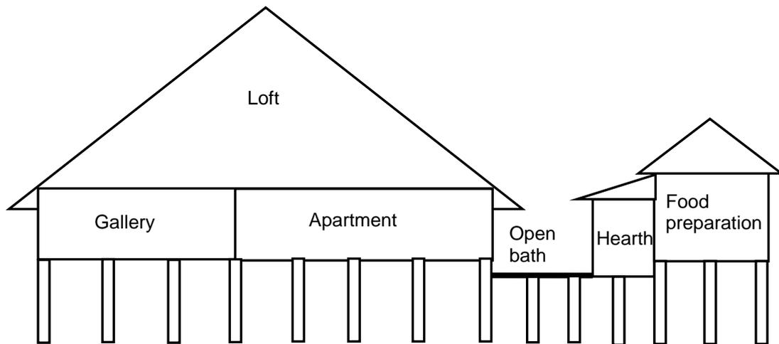
Fig.5. Cross section of the Merian Bedup longhouse before it was demolished in the year 2011. The roof was very high which provides a very good solar heat protection to the longhouse interior.
