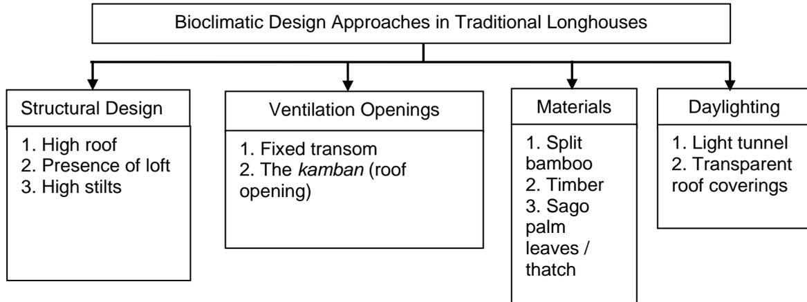
Fig. 1. Bioclimatic design approaches in traditional longhouses.
