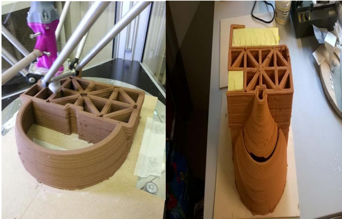
Fig 4. Clay 3D printing studies for components with specific design requirements (insulation assembly and light integration)
