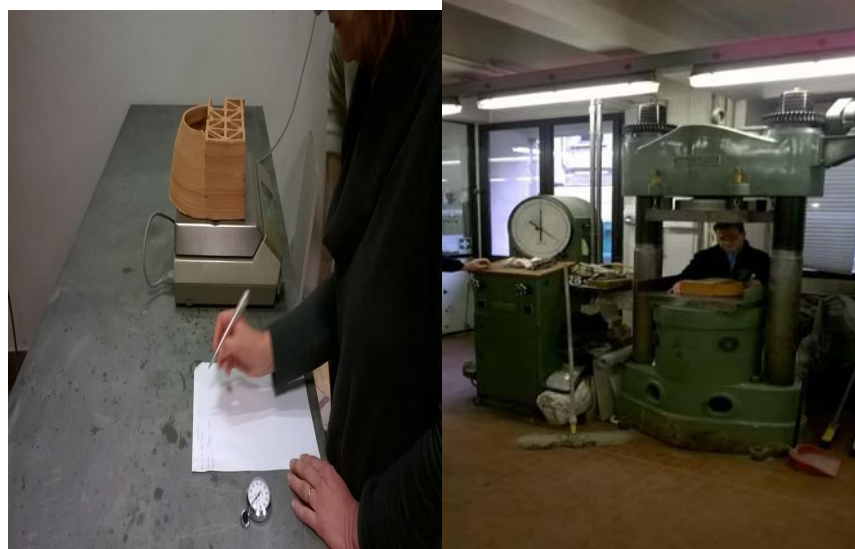
Fig 5: Absorption and structural testing of the 3D printed clay brick.
