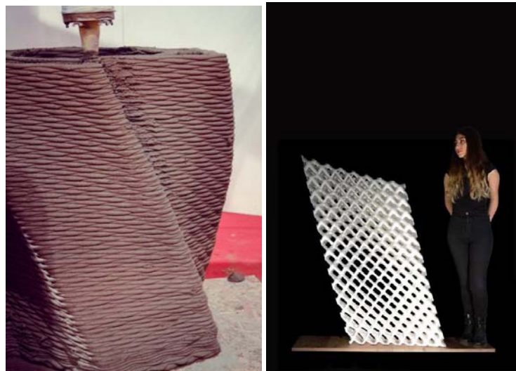
Fig. 6: Further developments on Additive Manufacturing techniques and applications within the research of ACTLAB. (a) 3D printing of a cement and resin based full scale complex form columns (b) cellular lattice based load bearing skin systems in PLA
