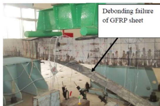
Fig.8 Debonding Failure of GFRP Sheet
