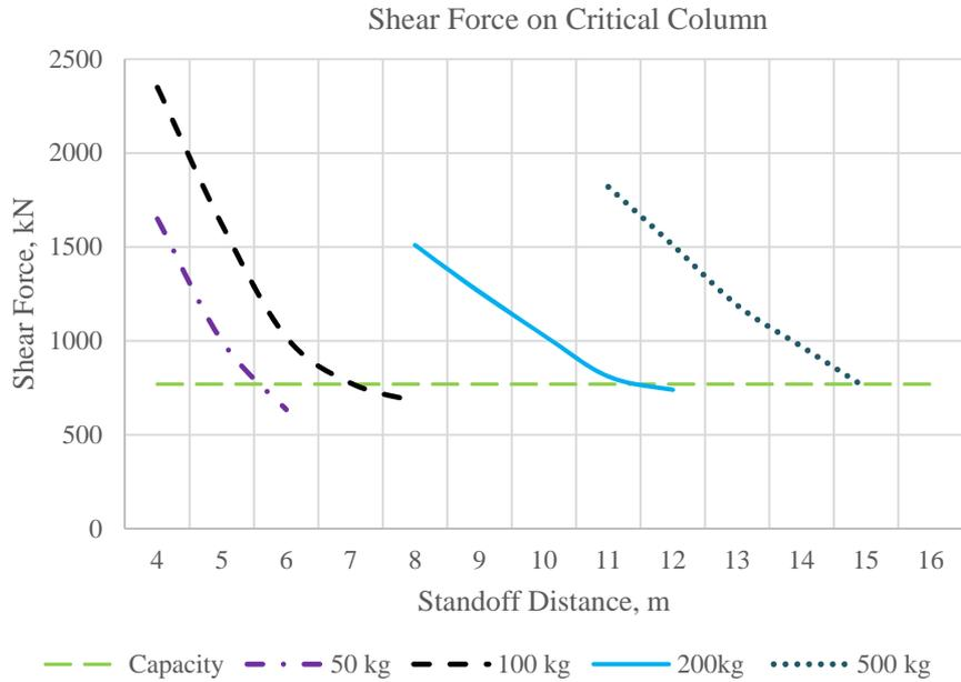
Fig. 2. Shear force on nearest column for various TNT blasts at different standoff distances
