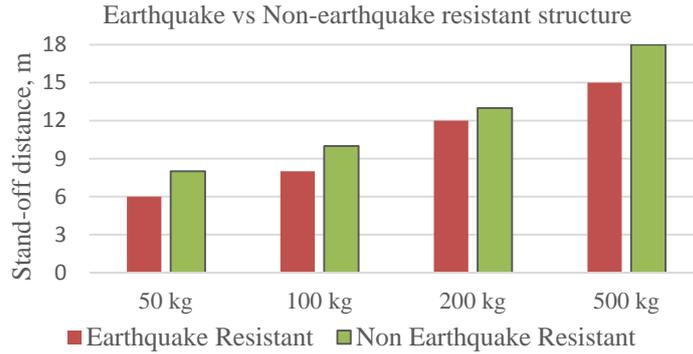
Fig. 4. Comparison of minimum standoff distances between Earthquake resistant and Non-earthquake resistant structures
