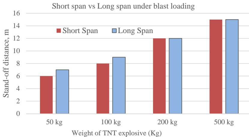
Fig. 5. Comparison of minimum stand-off distances when blast is acting on Short span vs Long span
