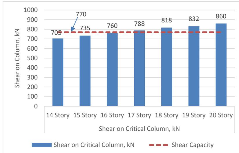
Fig. 6. Variation in shear force of selected column due to 100 kg TNT blast for structures with different stories.
