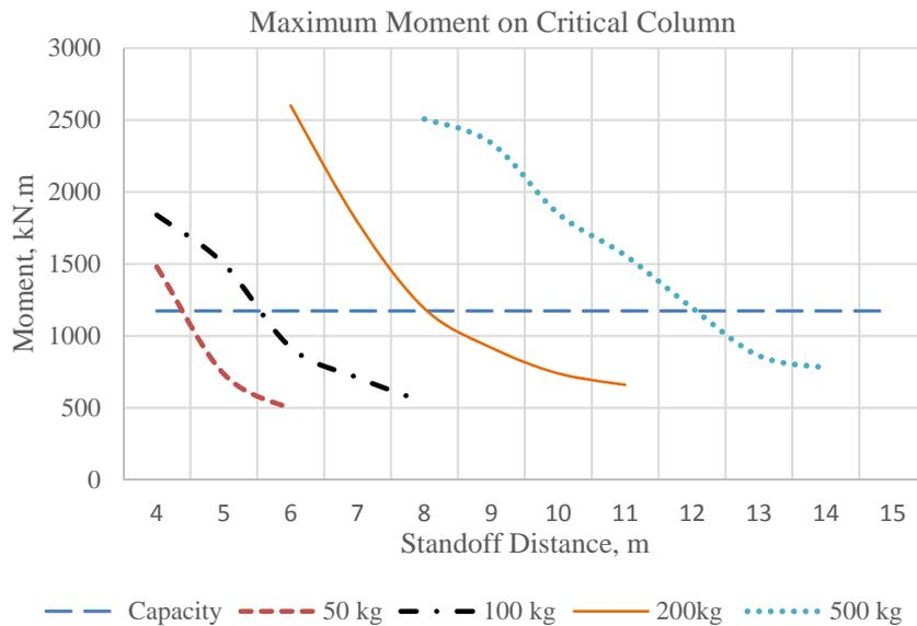
Fig. 2. Maximum moment in the nearest column for various TNT blasts at different standoff distances
