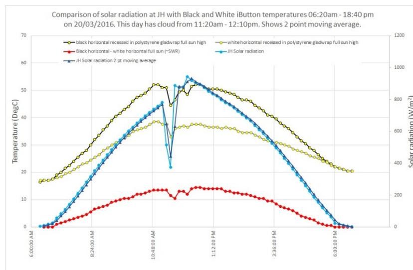
Figure 2 Comparison of solar radiation at JH with Black and White iButton temperatures 06:20am - 18:40 pm on 20/03/2016. This day has cloud from 11:20am - 12:10pm. Shows 2 point moving average.
