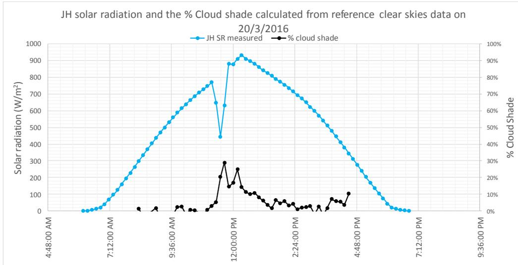
Figure 7 JH solar radiation and the % Cloud shade calculated from reference clear skies data on 20/3/2016.
