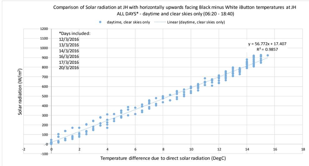
Figure 3 Solar radiation at JH versus horizontally upwards facing Black minus White iButton temperature at JH. ALL DAYS\* - daytime and clear skies only (06:20 - 18:40).
