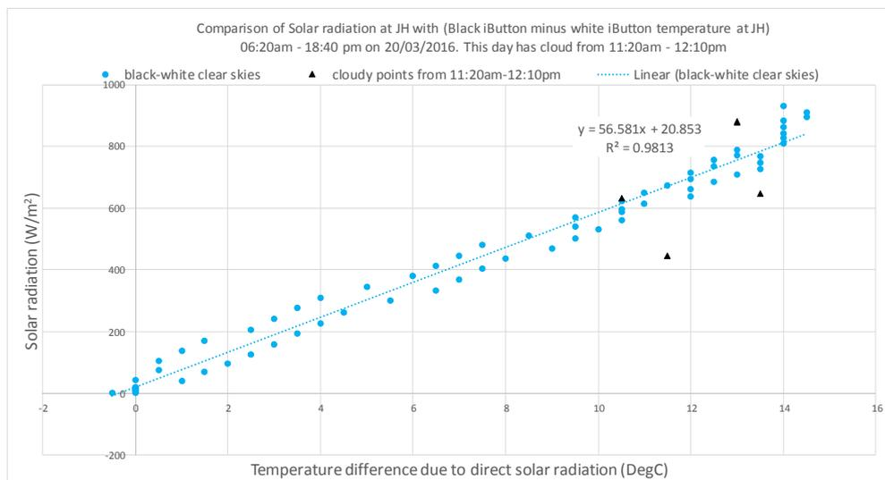
Figure 4 Solar radiation at JH versus horizontally upwards facing Black minus white iButton temperature at JH. 06:20am - 18:40 pm on 20/03/2016. This day has cloud from 11:20am - 12:10pm.
