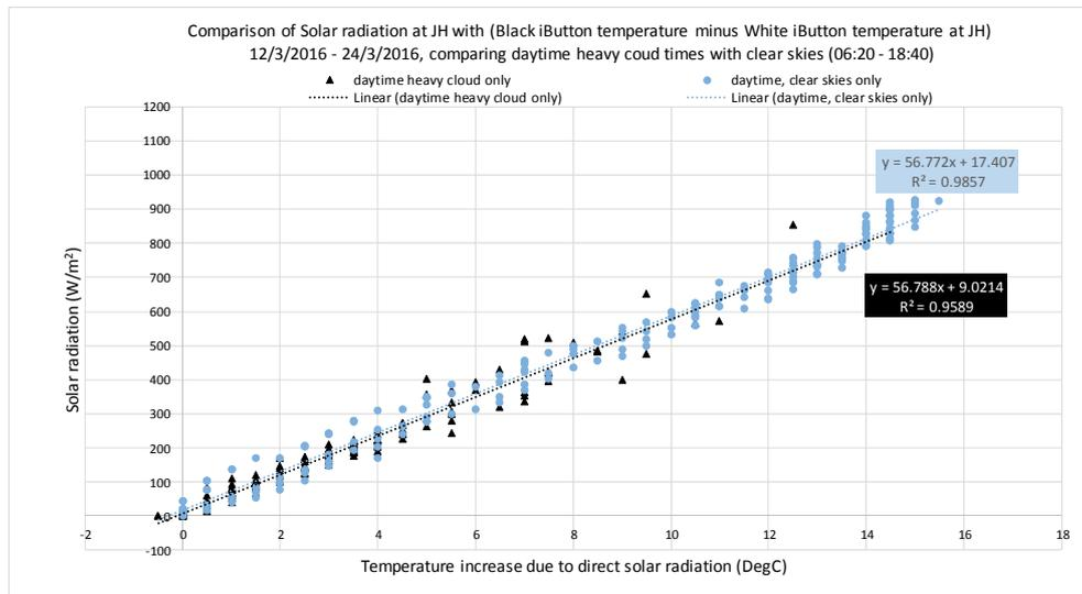
Figure 5 Solar radiation at JH versus (horizontally upwards facing Black minus White iButton temperature at JH) 12/3/2016 – 24/3/2016 clear skies only and 19/3/2016 and 23/3/2016 daytime heavy cloud only (06:20 - 18:40).
