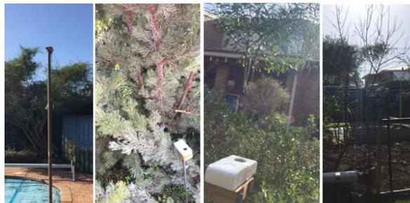
Figure 1 Images of the reference iButtons, iButtons under heavy, medium and light shade respectively.
