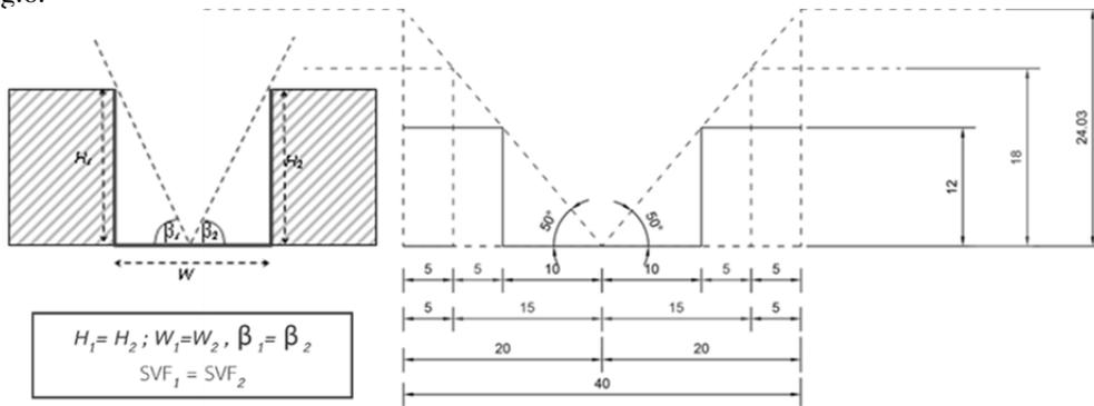
Fig. 5. H/W ratio calculation for uniform buildings.
