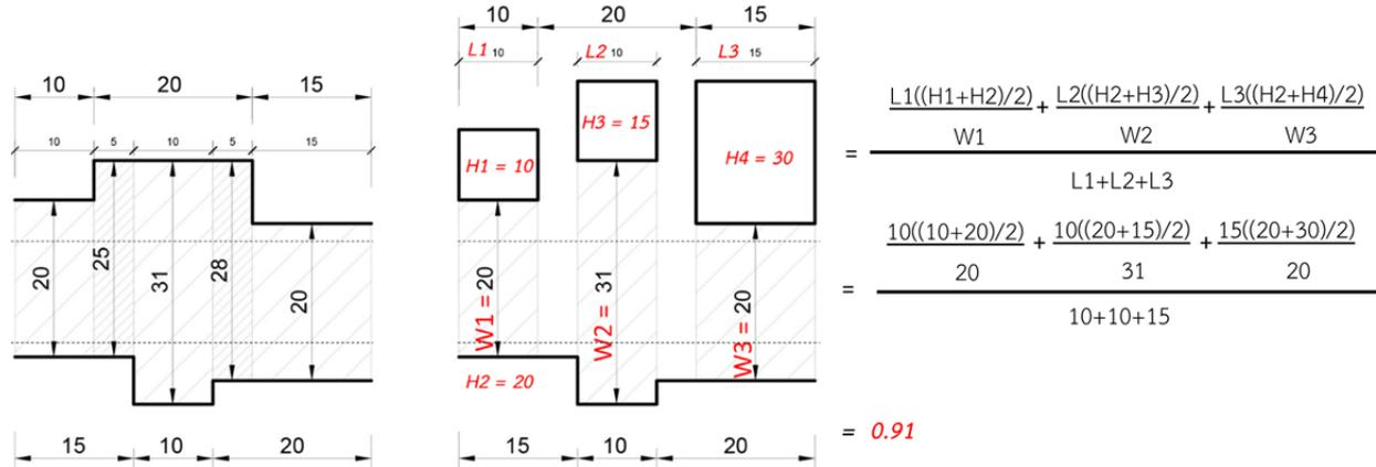
Fig. 7. An example of cross-sectional lines for finding H/W ratios on main road of Sala Daeng
