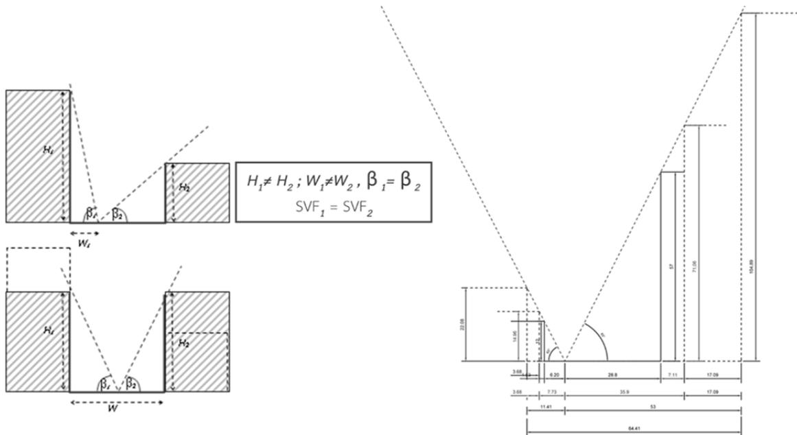
Fig. 6. H/W ratio calculation for non-uniform buildings.
