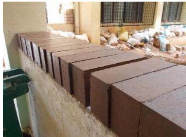
Fig. 7. Stacking of freshly prepared blocks
