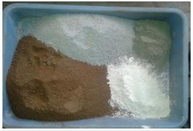
Fig. 5 Typical view showing weighed portion of various constituents used in the preparation of CSEB
