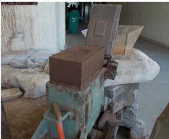
Fig. 6. Freshly ejected CSEB with MSW from Mardini press
