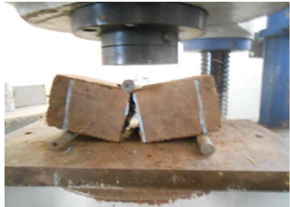
Fig. 11 Flexure test on block
