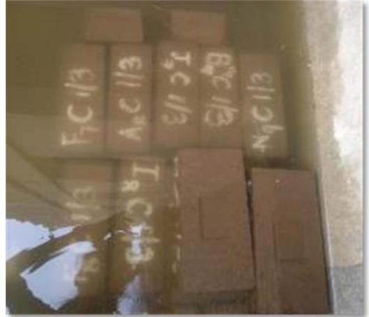
Fig. 9 View showing soaking of CSEBs in water before testing
