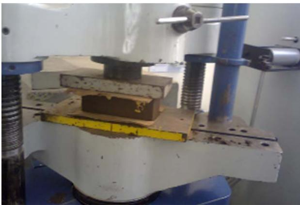
Fig. 10 Wet compression test on block
