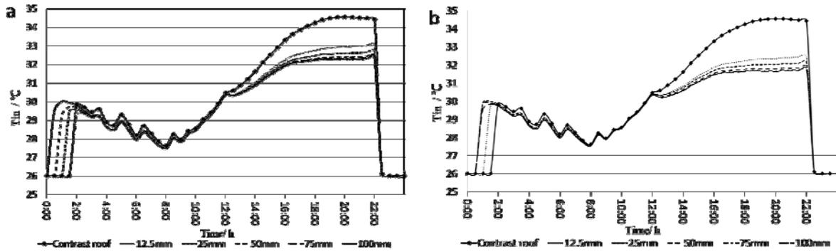
Fig. 4. Indoor hourly temperature for different insulation layer of insulation roof, (a) Inside insulation roof; (b) Outside insulation roof.
