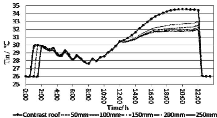
Fig. 6. Indoor hourly temperature for different aerated concrete layer of roof.
