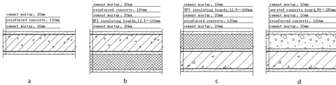
Fig. 2. (a) Contrast roof; (b) Light insulation roofing for inside; (c) Light insulation roofing for outside; (d) Heavy insulation roofing.
