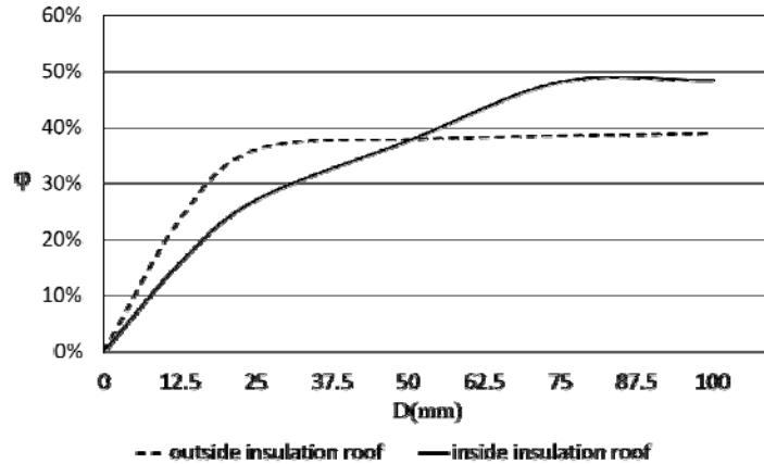
Fig. 5.The relative energy saving rate of the inside insulation roof.
