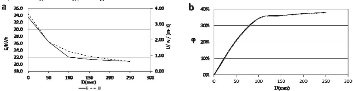
Fig. 7. (a)  $U$  and  $E$  for the roof with different thickness of aerated concrete; (b)  $\varphi$  for the roof with different thickness of aerated concrete.
