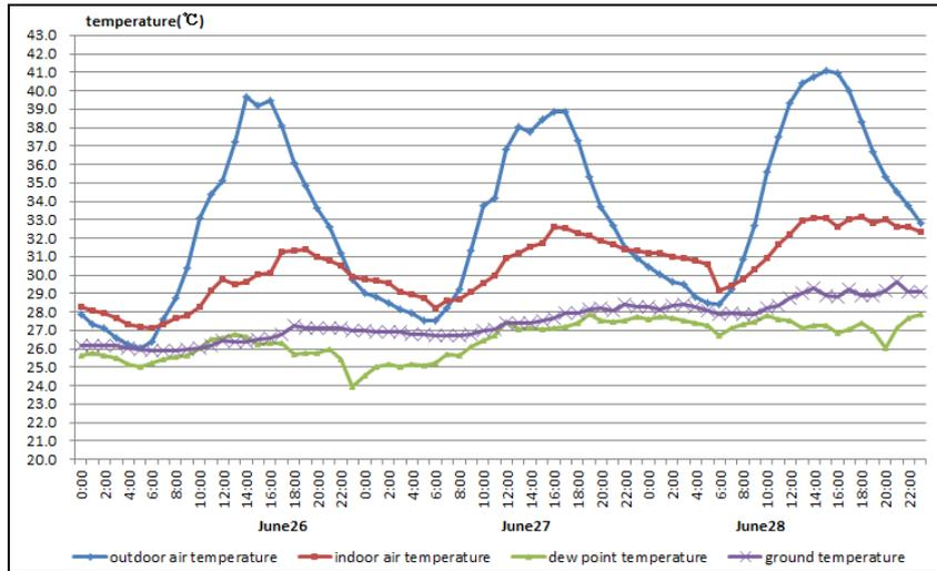
Fig.6. Relationship between indoor temperature and ground temperature from 26th to 28th in June
