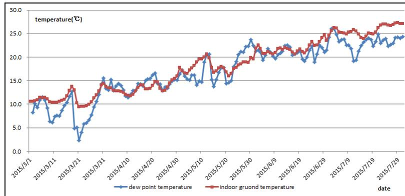
Fig.4. Contrast curve of indoor air dew point temperature and ground temperature of rural residence
