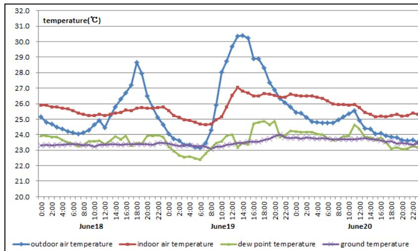
Fig.5. Relationship between indoor temperature and ground temperature from 18th to 20th in June
