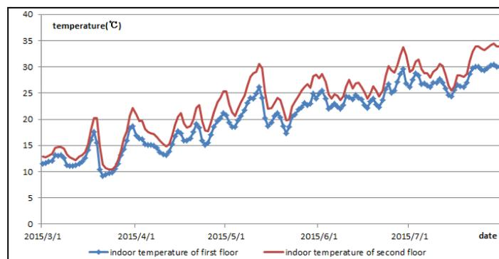
Fig.3. Contrast curve of indoor air temperature change between the first floor and the second floor of rural residence
