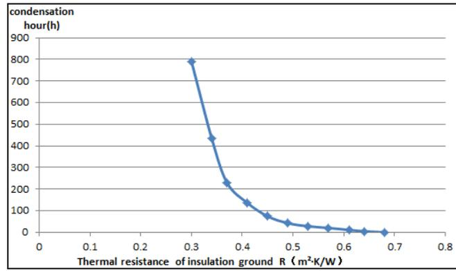
. Fig.8. Relationship between condensation hour number and thermal resistance of insulation ground.
