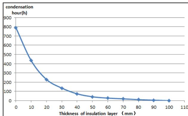
Fig.7. Relationship between condensation hour number and thickness of insulation layer.
