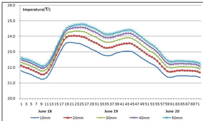
. Fig.9. Comparison of ground temperature and ordinary cement ground temperature in different thickness from 18th-20th in June.
