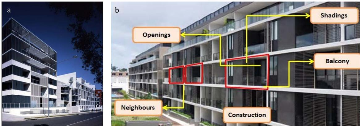
Fig. 3. examples of single-sided façade design commonly used in Sydney mid-rise residential buildings: (a) Rhodes residential development[15]; (b) illustration of key design variables [16]
