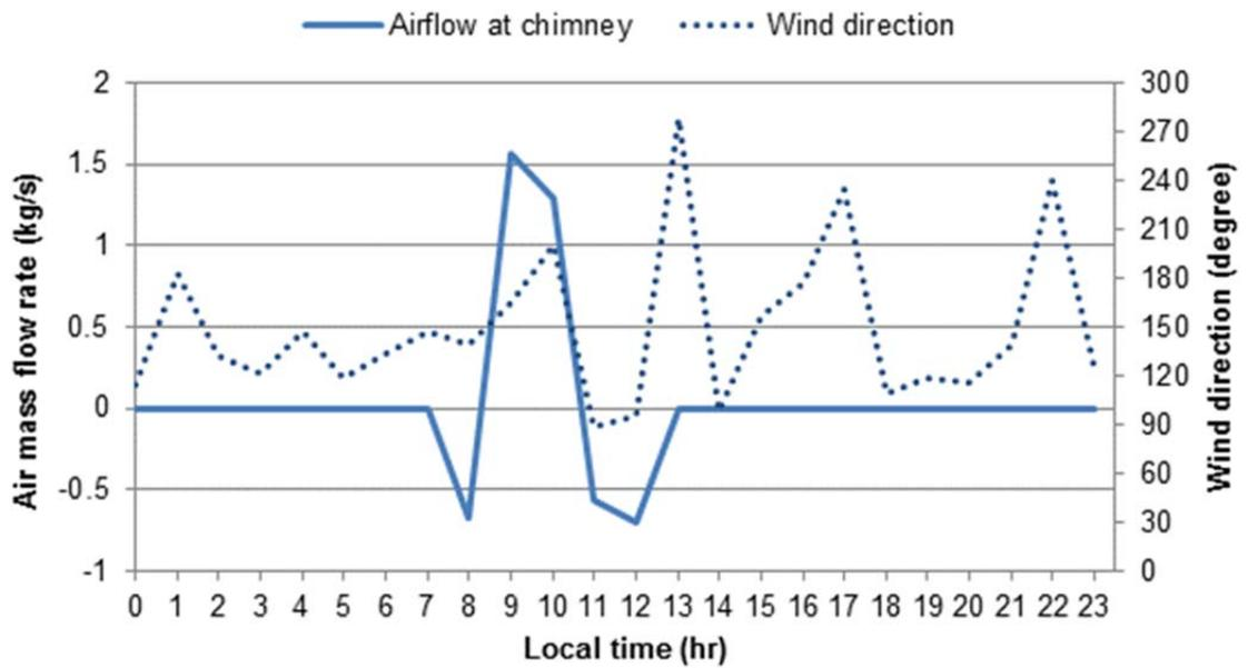
Fig.10. Predicted airflow rate at the solar chimney and the corresponding wind direction on 19th Jan 2012 (Wind direction: 0° refers to North, +Ve indicates air flow into the atrium )
