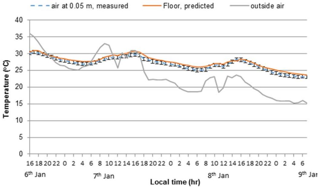
Fig. 5. Comparison of predicted floor temperature with measured air temperature near the floor in a sealed atrium with closed roof shade (Jan 6-9 2012)
