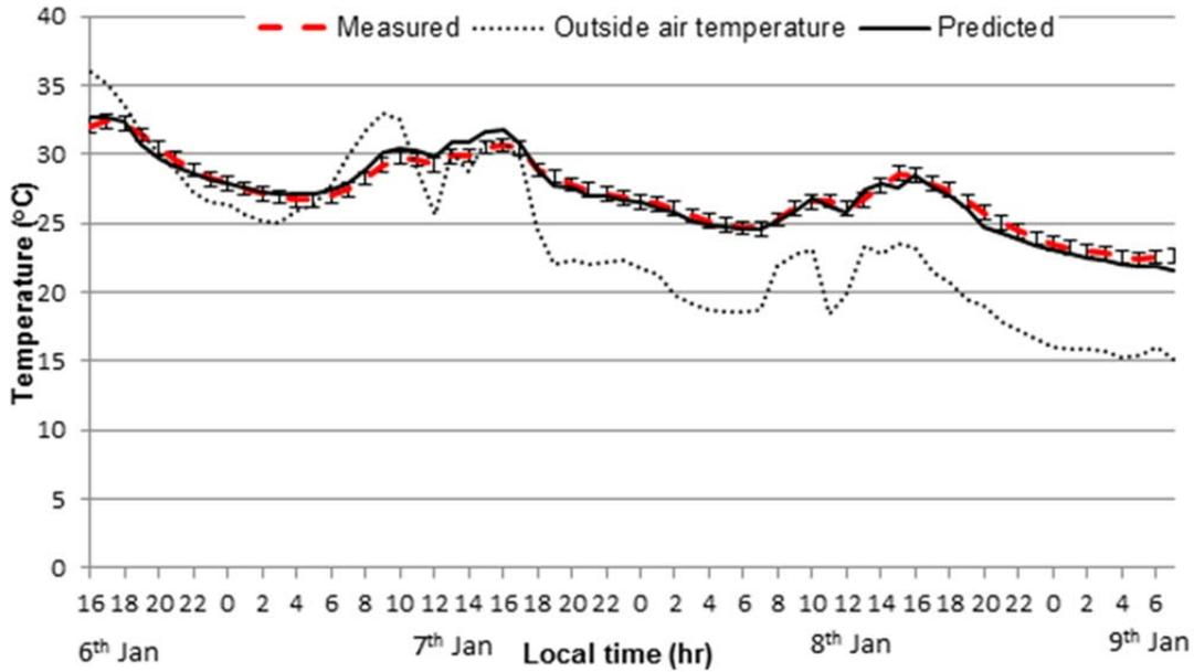
Fig. 4. Comparison of average air temperatures in a sealed atrium and roof shades closed (Jan 6-9 2012)
