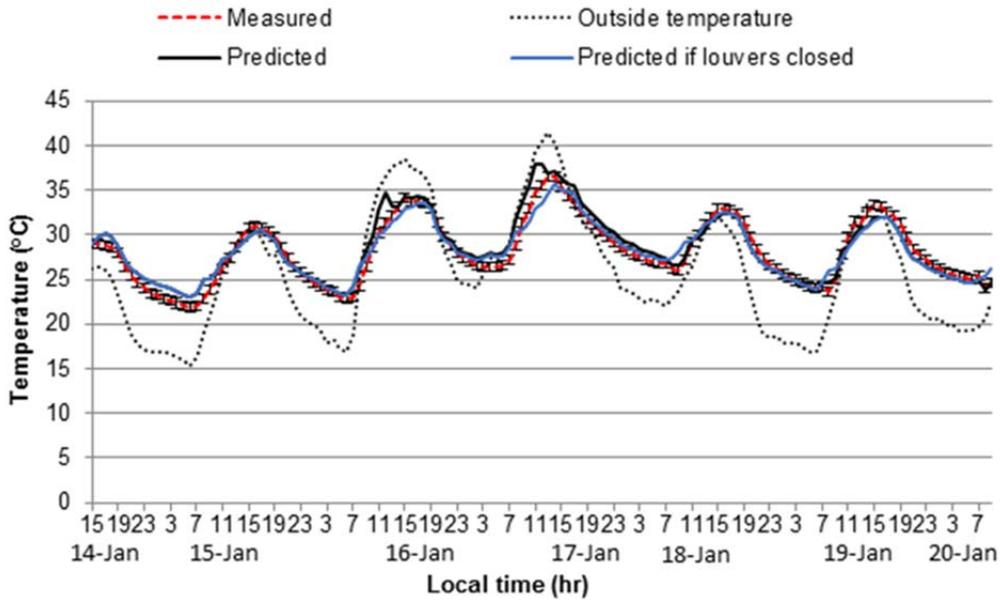
Fig. 8. Comparison of predicted and measured atrium air temperature (roof shade closed; Jan 14-Jan 20, 2012)
