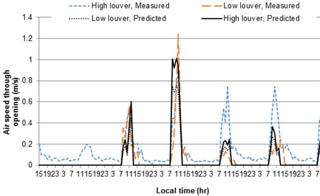
Fig. 9. Comparison of predicted and measured airflow rates through openings in the atrium (roof shade closed; Jan 14-Jan 20, 2012)
