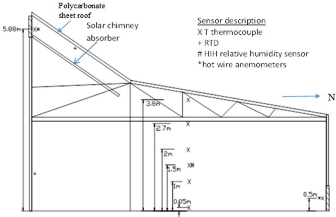
Fig. 1. Cross-section of the atrium showing the exact location of sensors
