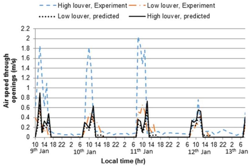
Fig. 7. Airflow rates comparisons across the low and high level louvers: predicted and measured, roof shade open (Jan 9 - Jan 13 2012)
