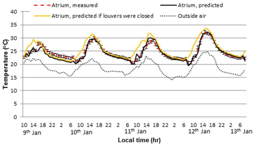
Fig. 6. Comparison of average atrium air temperature with the roof shades open (Jan 9-Jan 13, 2012)
