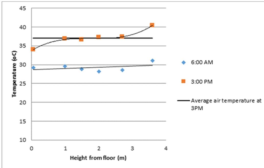
Fig. 3. Atrium air temperature with height; sealed building with roof shades closed, Jan 2, 2012; maximum outside temperature 43°C
