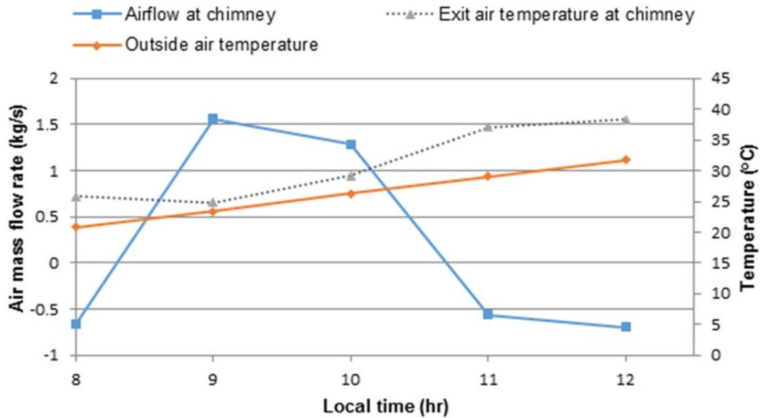
Fig.11. Predicted flow reversal and exit air temperature from the solar chimney on 19<sup>th</sup> Jan 2012
