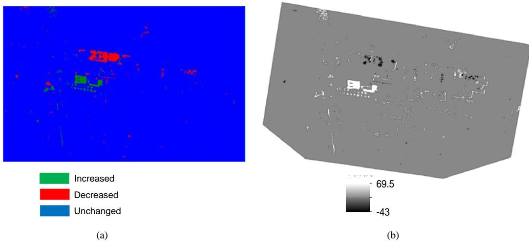
Fig. 5. Change detection results: SVM (a), DSM differencing with  $\gamma=4$  (b)
