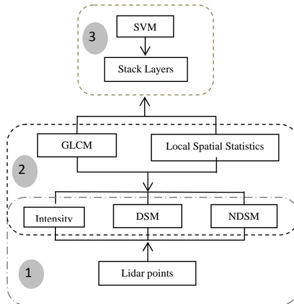
Fig. 2. The method of applying SVM for building classification and change detection using airborne lidar data
