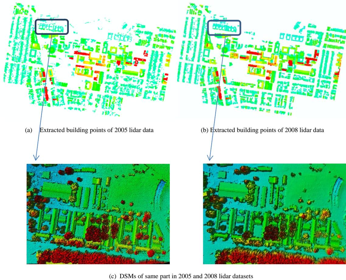
Fig. 4. Inconsistent results of building classifications for 2005 and 2008 datasets (a and b), the DSMs (c) of the corresponding areas from careful visual inspection for existence of any building change between 2005 and 2008 datasets.
