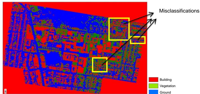
Fig. 3. The problem of misclassification between roads and buildings in sloping terrain of UNSW dataset using SVM method
