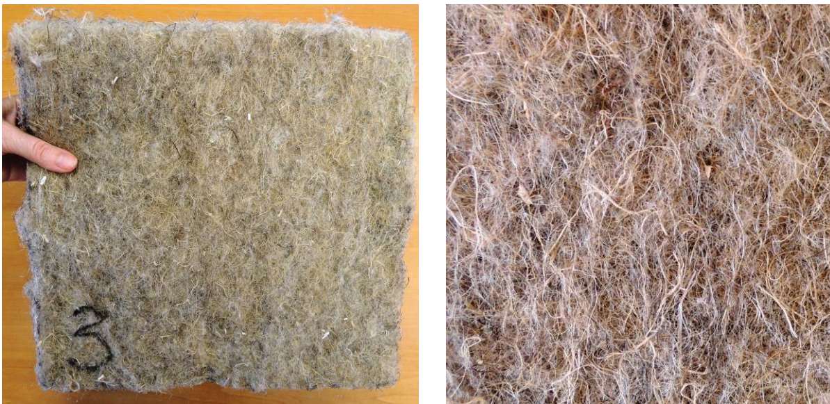
Fig. 1: A sample of the hemp-based insulation and his structure
