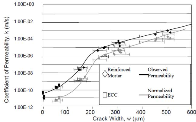
Fig. 2. Coefficient of permeability vs. crack width for ECC and reinforced mortar [10]
