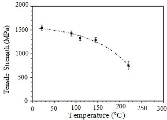
Fig. 1. Tensile strength of PVA fiber at various temperatures [9]
