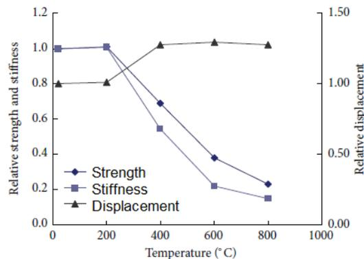
Fig. 3. Compressive strength, stiffness, and displacement at peak load with temperature (Shang and Lu, 2014)
